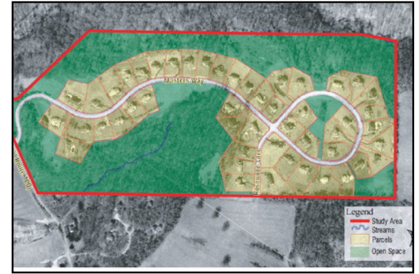
Reserves at Chaddsford Year approved: 1993 Housing: 55 single-family units Tract Size: 132.77 acres Open space: 59% (78.33 acres) Gross Density: 1 unit per 2.4 acres Parcel Size (Estimated): 29,000 - 34,000 SF
