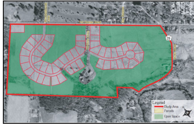
Pickering Glenn Conservation Subdivision Year Approved: 2000 Housing: 49 single-family units Tract Size: 115.22 acres Open Space: 63% (72.56 acres) Gross Density: 1 unit per 2.35 acres Parcel Size (Estimated): 25,000 - 30,000 SF
