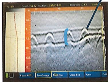
Picture 11: The above data screenshot shows a potential void found in Area C. This data screenshot shows a high amplitude negative response in the data that is consistent with those of a void.
