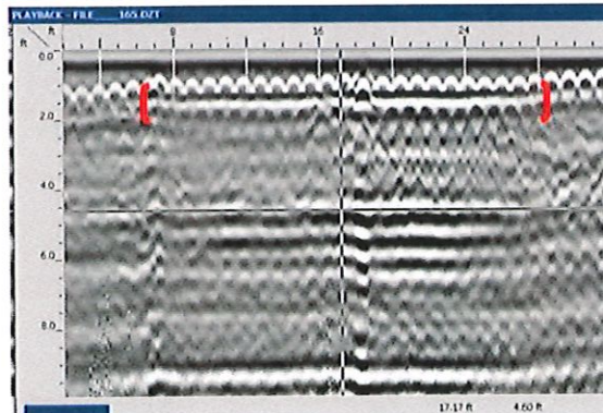
Sample GPR data screenshot showing a void that was verified to exist directly below a concrete slab that was reinforced with rebar.
