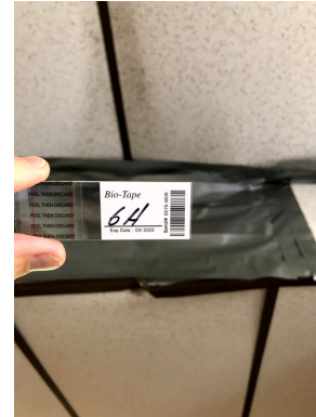
26. Stained Ceiling Panel - Location of Surface Sample 6H (Living Room)
