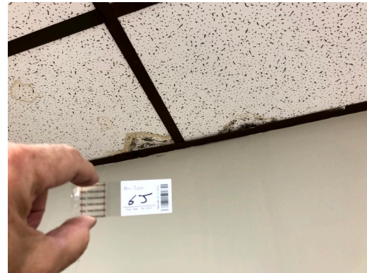
26. Stained Ceiling Panel - Location of Surface Sample 6H (Living Room)
