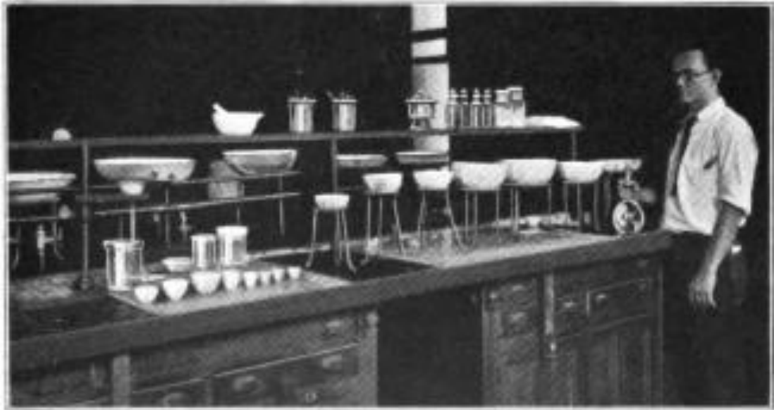
PLATE NO. 5. BROMIDE CRYSTALLIZING SYSTEM.
